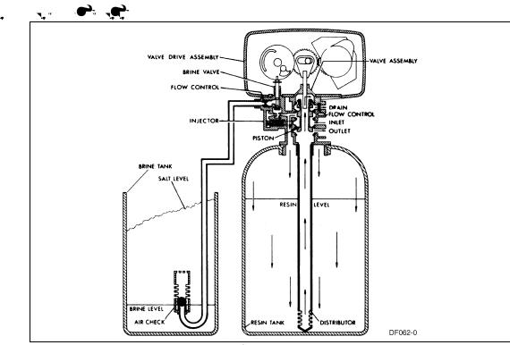
Figure 10: Settling Rinse Position
