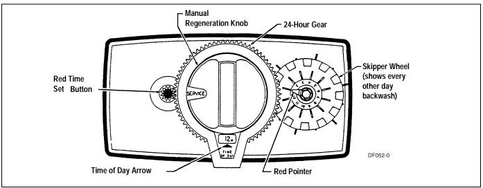
Figure 2: Model 5600 Backwash Filter Control
